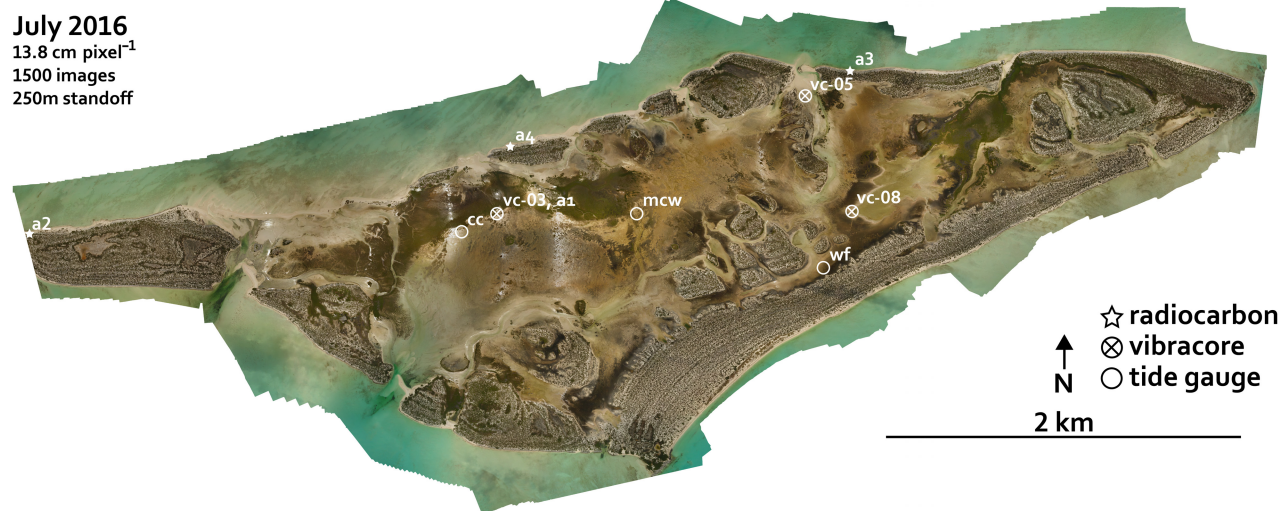
Fig. 2. Orthomosaic of Little Ambergris Cay produced in July 2016 using a DJI Phantom 4 Pro uncrewed aerial vehicle (UAV) with a 12-megapixel camera. More than 1500 RGB images were collected during 13 separate flights over seven days, yielding 13.1 cm pixel -1 resolution. Photogrammetry was conducted in Agisoft Photoscan. White streaks represent specular reflection of sunlight on shallow water. The images are not radiometrically corrected. Locations of vibracore measurements (Fig. 17) and tide gauge measurements (Fig. 3C) are shown.
